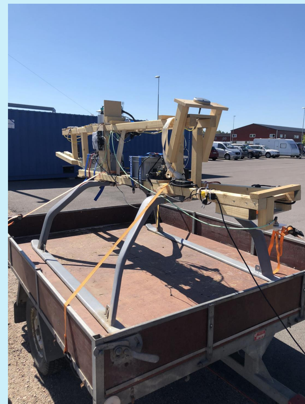
Figure 1. Experimental setup. The navigation sensors are attached to the wooden UAV test chassis.
