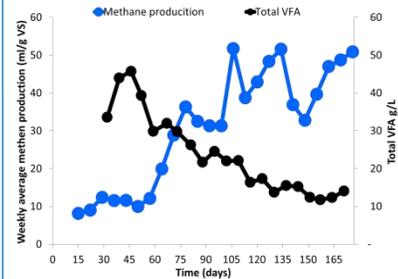
Figure 2) Methane production and VFA concentration during the plug-flow experiment in pilot-scale.
