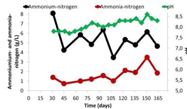
Figure 3) Ammonium- and ammonia nitrogen content in the digestate out from the plug-flow reactor.
