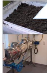
Figure 1) The digestate and the plug-flow reactor in pilot-scale that was used for the experiment
