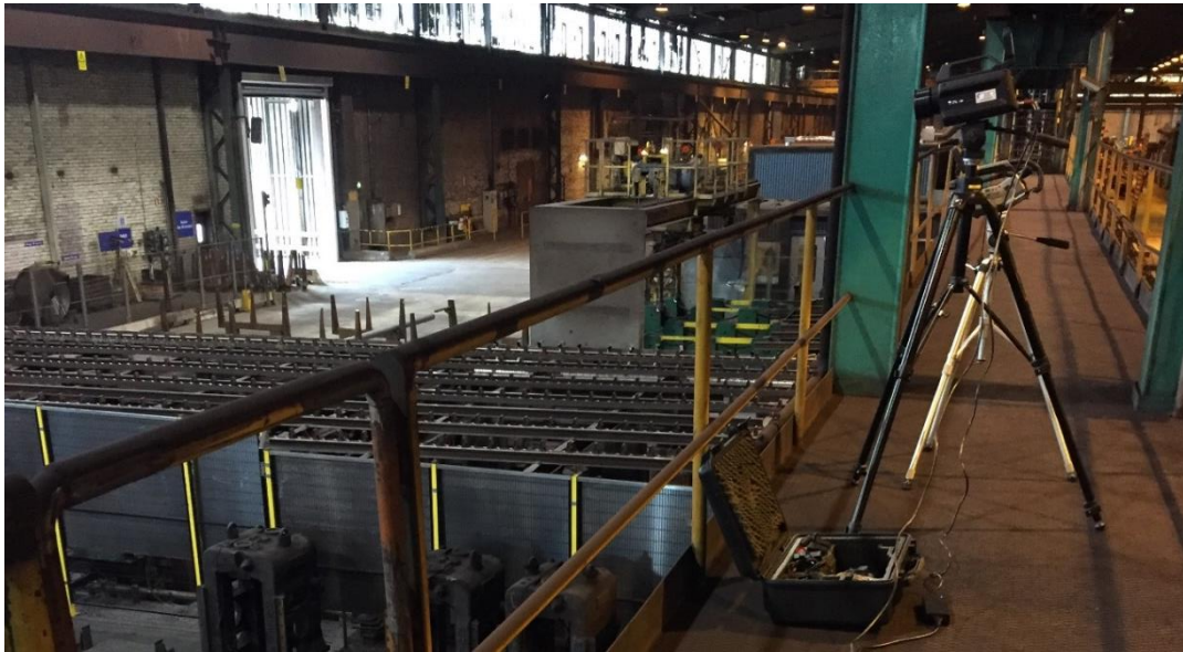
Figure 65 Position of camera on top of the straightening and cooling bed process.
