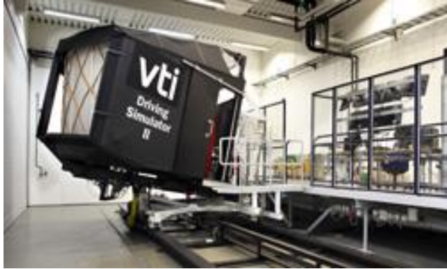
Sim II, truck/fire engine moving base
