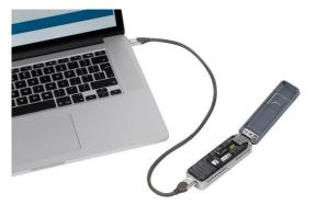
Illustration of the handheld MinION. (With kind permission from Oxford Nanopore Technologies)
