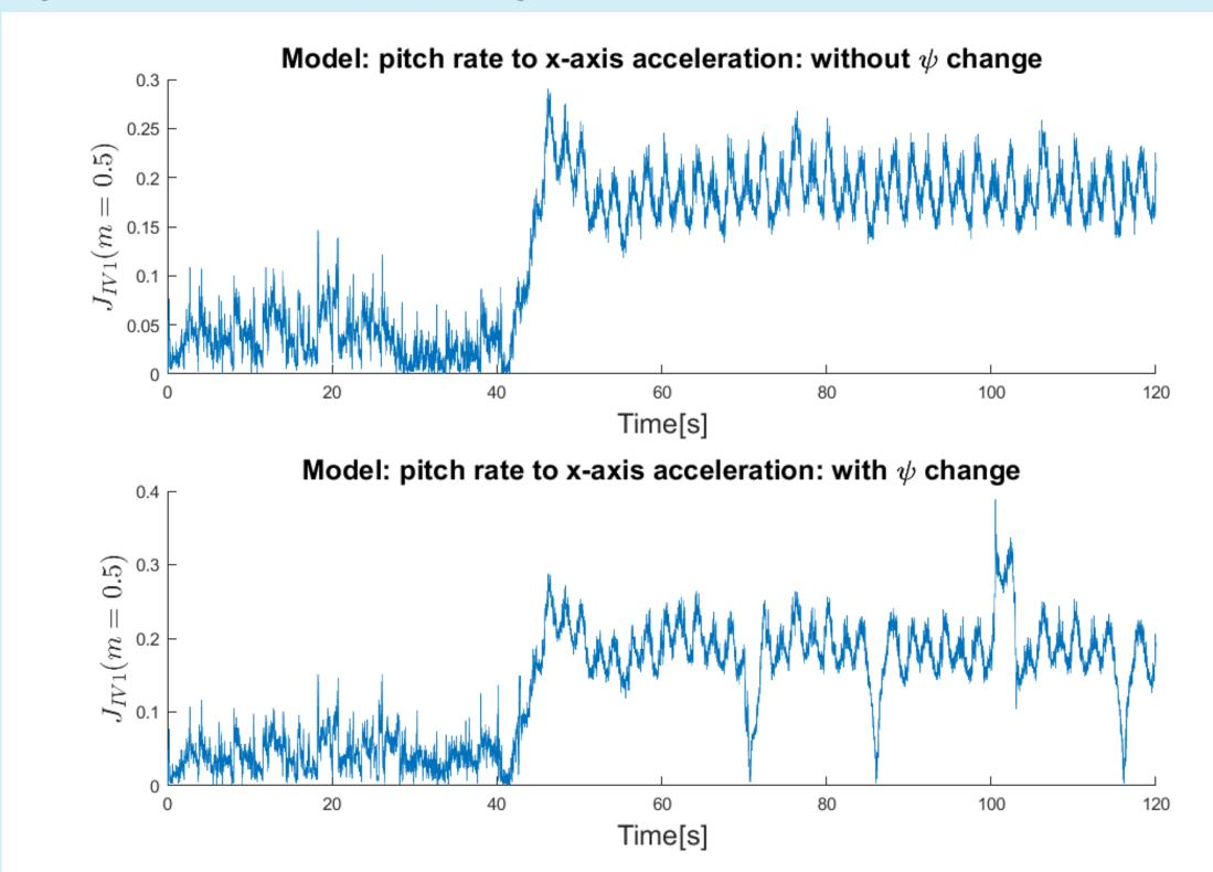
The payload changes are detected using the IV cost function with and without course angle variation.
