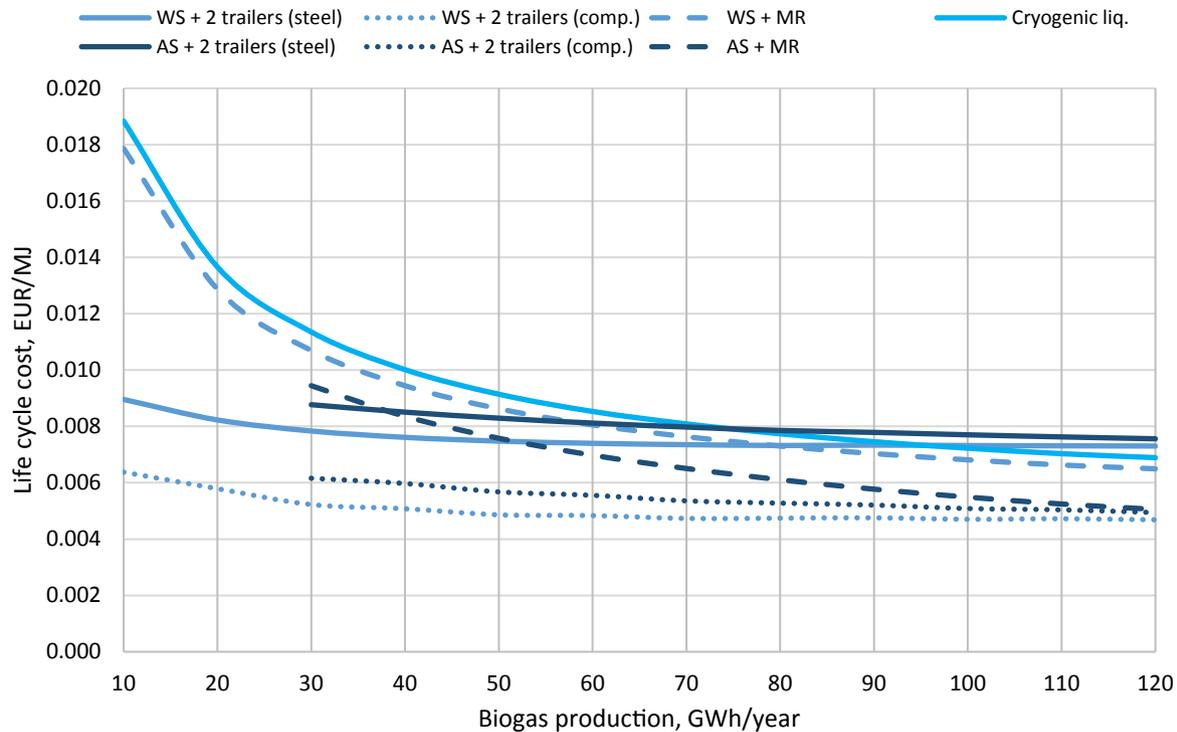
Fig. 4. Life cycle cost of scenarios for upgrading, liquefaction and distribution of biogas as a function of annual production capacity, for a distribution distance of 100 km.
