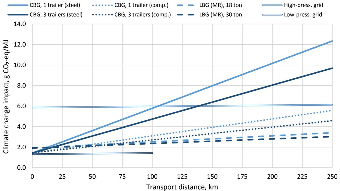
Fig. 6. Climate change impact for CBG pathways as a function of transport distance from production site to customer area.
