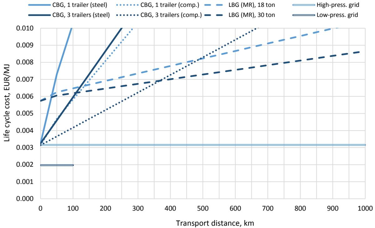
Fig. 7. Life cycle cost for CBG pathways as a function of transport distance from production site (120 GWh/a) to customer area.
