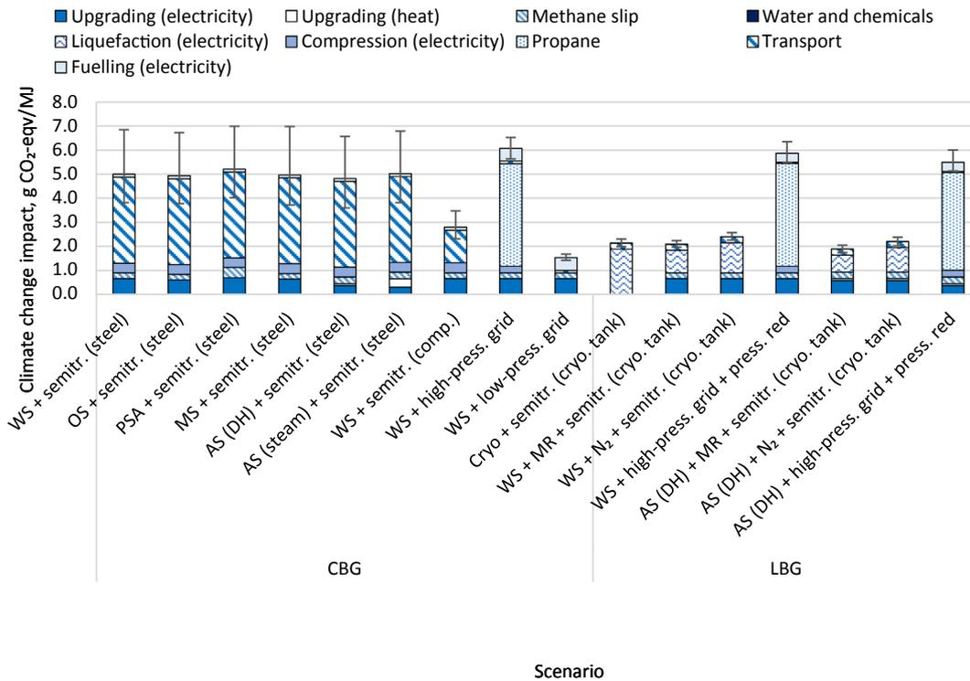
Fig. 3. Climate change impact of scenarios for production and distribution of compressed and liquefied biogas. “Transport” includes distribution over a distance of 100 km. The error bars indicate the 95% confidence interval for environmental impact.
