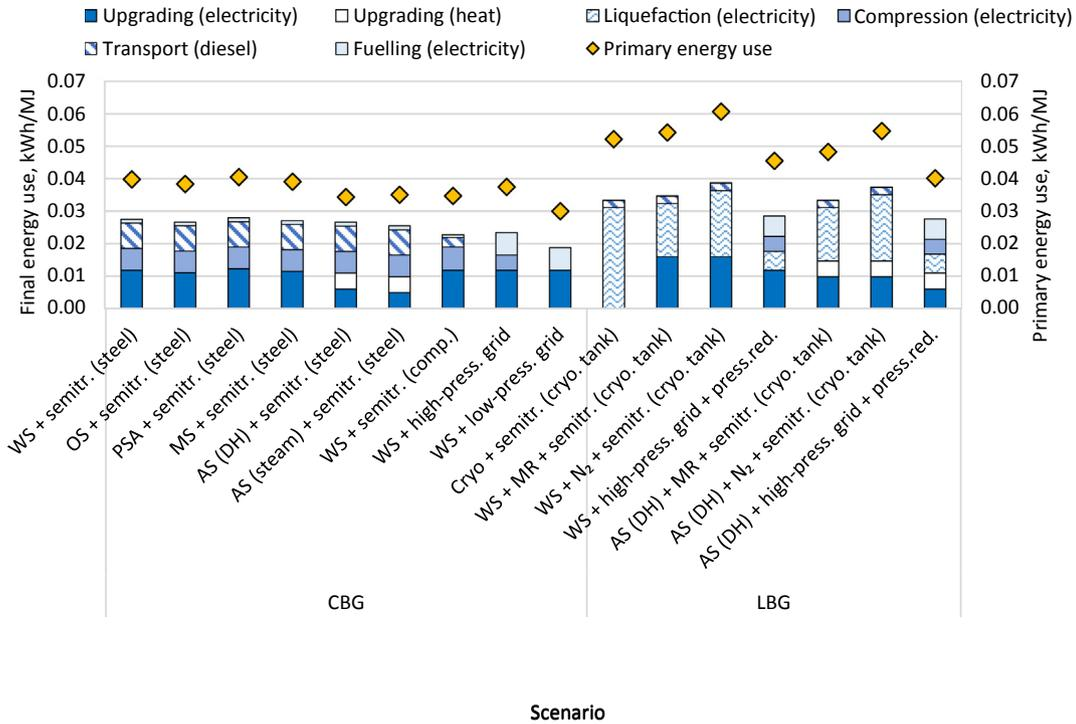
Fig. 2. Final energy use (bars) and primary energy use (diamonds) of scenarios for production and distribution of compressed (CBG) and liquefied biogas (LBG).
