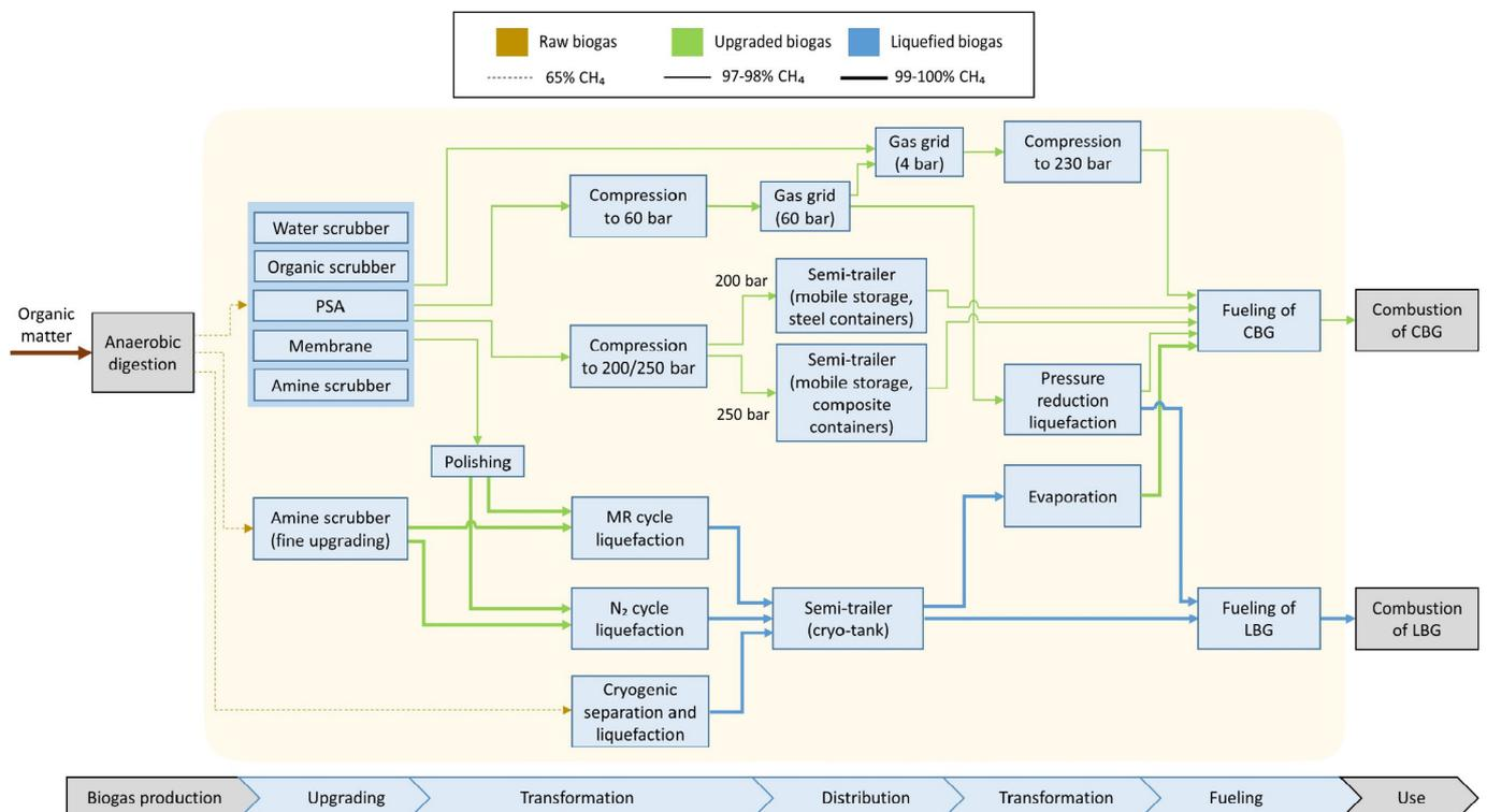
**Fig. 1.** Schematic view of the modelled scenarios for upgrading, liquefaction and distribution of biogas. Going from the left to the right, each of the indicated pathways represent a possible scenario from biogas production to end user. The color and weight of the lines indicate the state and methane content of the gas.
