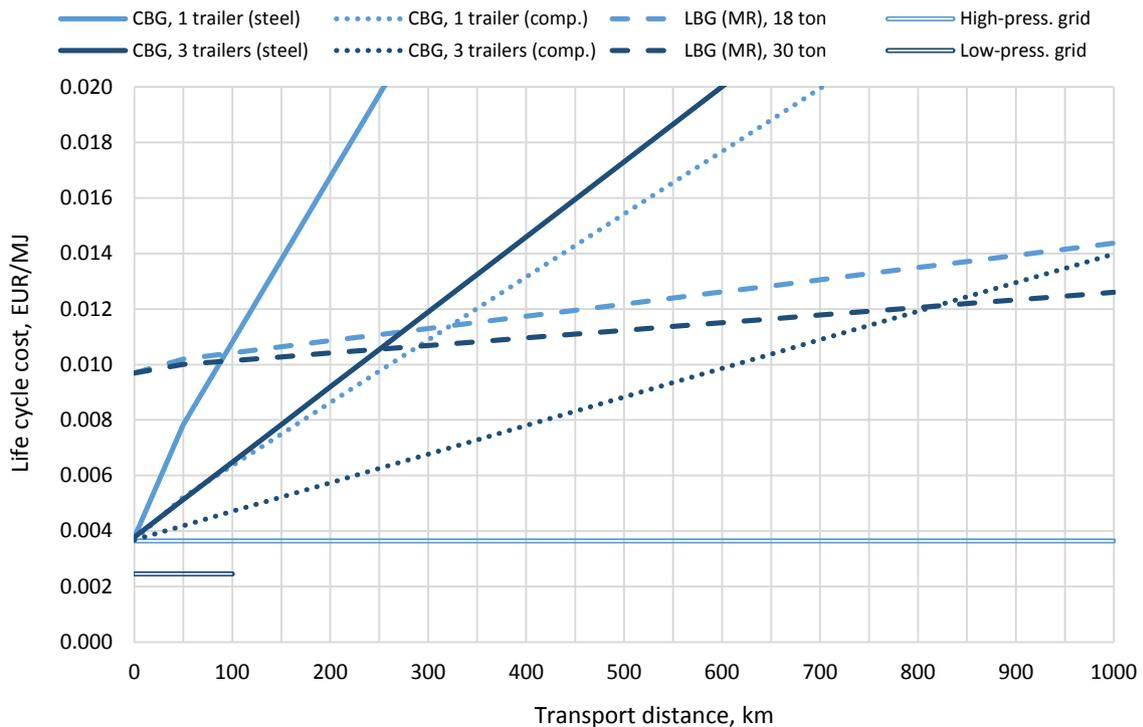
Fig. 8. Life cycle cost for CBG pathways as a function of transport distance from production site (30 GWh/a) to customer area.
