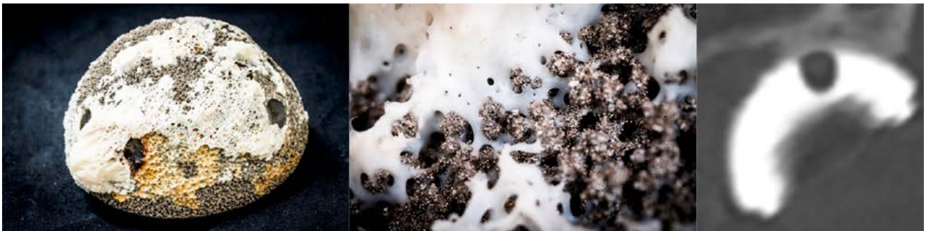
Figure 1. Retrieved acetabular cup implant (left) with newly formed bone integrated with the porous surface of the implant (middle, with courtesy of Thor Balkhed, Linköping University) and the clinical CT image of the cup acquired using conventional CT before revision surgery (right). Due to the limited spatial resolution, the visibility of the interface between the bone and the implant is not good enough to evaluate whether there is adequate osseointegration.
