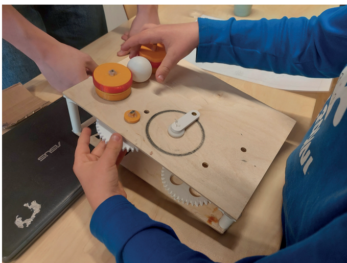
3D Printed Gear System
