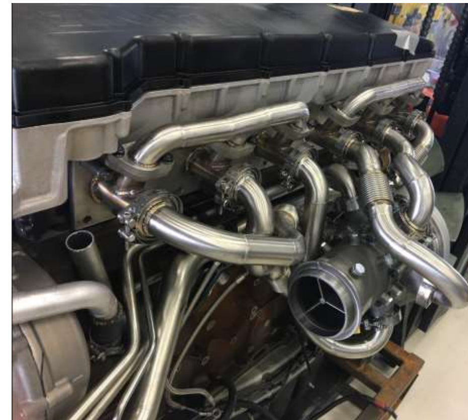
Figure 65: "Six-sector" axial turbine stage. From Paper 7.
