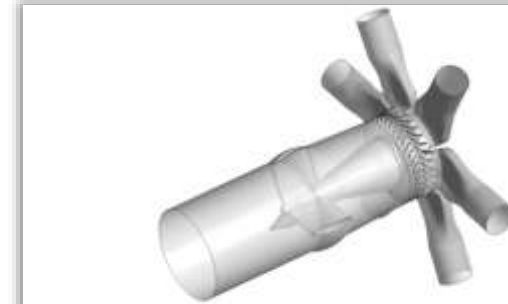
Figure 65: "Six-sector" axial turbine stage. From Paper 7.
