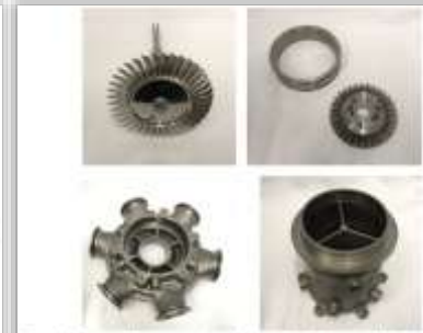
Figure 66: Prototype turbine stage, near upper left, lower and axial paper right, turbine housing (lower left) and lower housing (lower right). From Paper 8.
