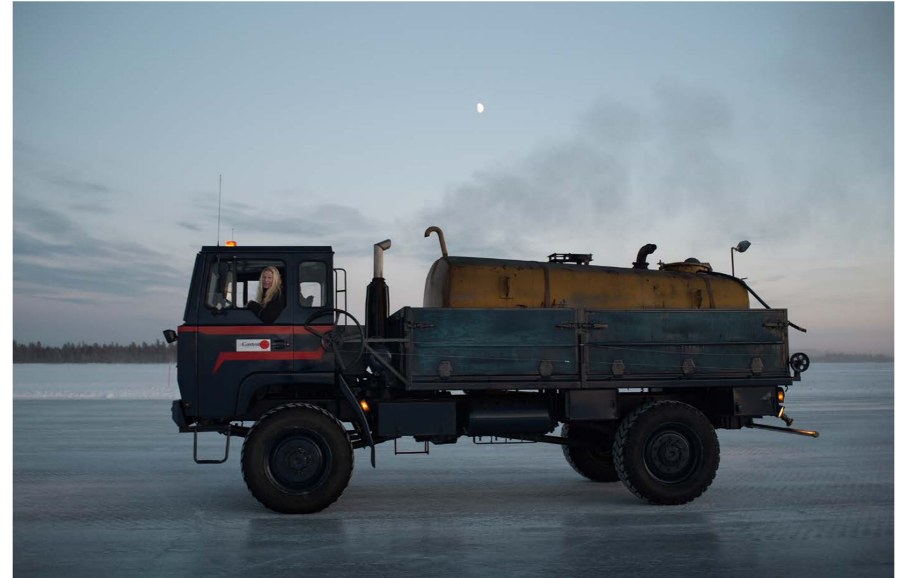
Figure 9. A still from the film by Camilla Andersen showing Åse in her truck, which is used to spread water thinly on the ice to make it more slippery for brake-testing. Camilla's cinematic choices were also a key part in weaving together the themes from fieldwork with the interview material, which we edited together collaboratively.
