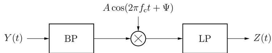
The two filters are ideal, with cut-off frequencies chosen so that the useful signal passes the filter unchanged. We assume full synchronization, i.e.  $\Psi$  is completely known at the receiver.
